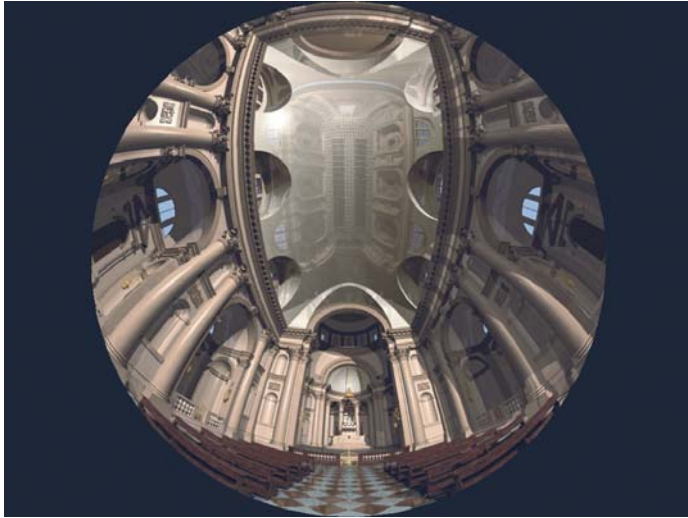
Figure 6. Fisheye image shown in 6a is applied as an OpenGL textured mesh in 6b. Each mesh node in 6b is represented by (x,y) coordinate in normalized projection plane coordinates, a (u,v) texture coordinate that relates to the fisheye image, and an intensity value that can compensate for the variable light path length.
