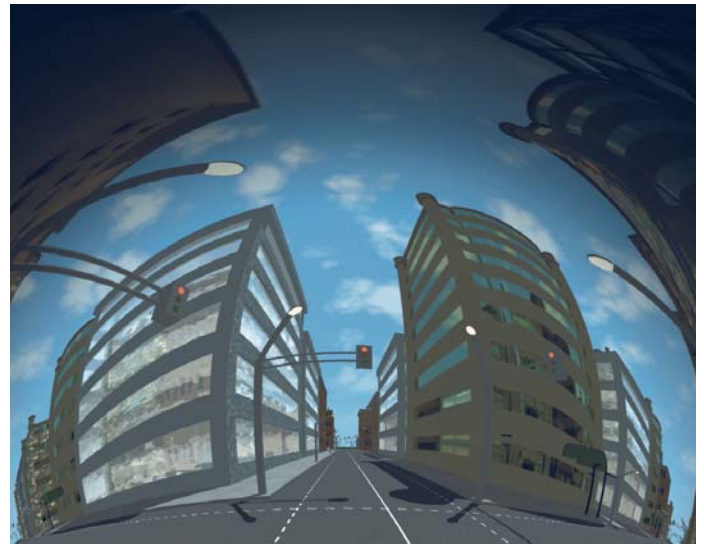
Figure 7. 7a shows the warped appearance of the four texture regions and mesh outline as used by real-time OpenGL applications. The textures are derived from 4 virtual cameras each with the face of a cube as the projection plane. 7b is a single frame from a real-time driving simulator using the warped texture meshes in 7a.
